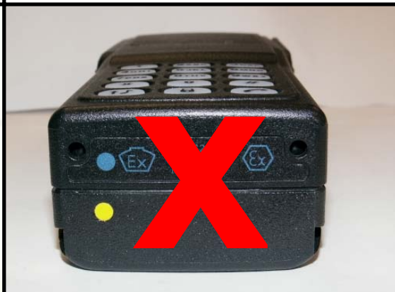
Fig 6. Cenelec Radio with incorrect ATEX Battery
